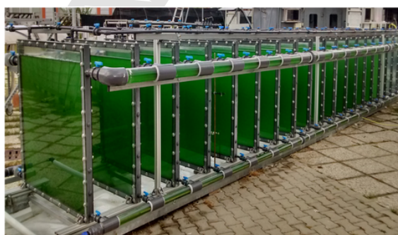
Fig. 10. The flat panel PhotoBioReactor (PBR) system (maximum working volume 1300 L) is composed of 20 vertical parallel plates 50 L, 1150 × 1150 × 50 mm (W × H × D), in direct communication with each other, left. Daily variation of maximum quantum efficiency of PSII photochemistry ( F_v/F_m ) and effective photochemical quantum yield of PSII ( \Delta F/F_m' ) right. Data are shown as mean \pm SD, n = 3.
